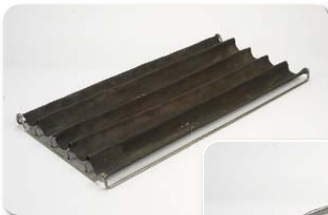
Filet encrassé Clogged filet
